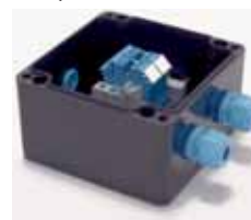
Art.-Nr. WZX189EX Terminal enclosure Ex i (Sensors) Marking: ⊕ II 2G Ex ia IIC T6 ⊕ II 2D Ex tD A21 T+85°C IP66 Equipment: 3 cable glands, 1 blind plug, 7 terminal blocks Dimensions (LxWxH): 122 x 120 x 90 mm
