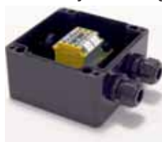
Art.-Nr. WZX188EX Terminal enclosure Ex e (mains) Marking: ⊕ II 2G Ex e IIC T6 ⊕ II 2D Ex tD A21 T+80°C IP66 Equipment: 2 cable glands, 2 blind plugs, 6 terminal blocks Dimensions (LxWxH): 122 x 120 x 90 mm
